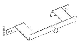
**ASK73.1** This bracket provides an extended antirotation pin that allows two ES142 actuators to directly drive a single damper shaft. For use with two and three–position actuators.
